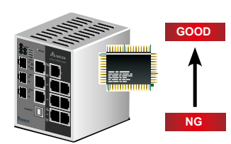
CPU malfunction = 6 seconds = Auto Reset
